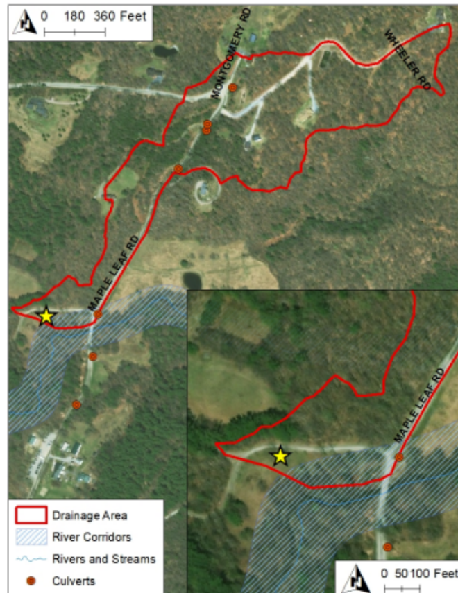
Figure 16. The drainage area for the proposed BMP is shown in red for the Maple Leaf Rd (1) site. The proposed BMP location is shown with a star.
